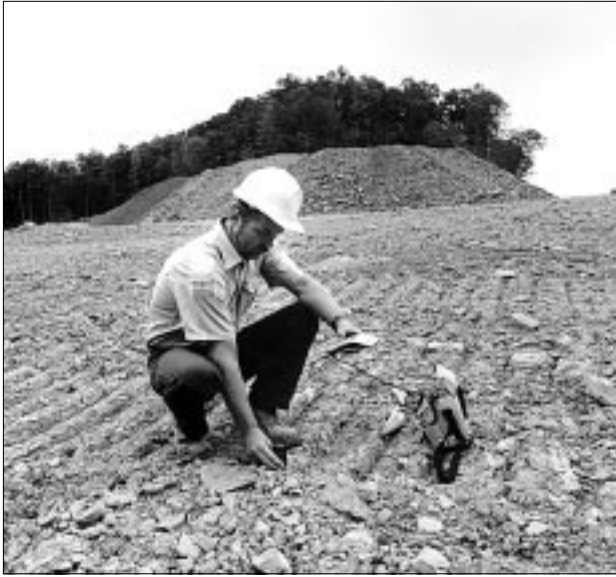
This mine inspector is checking soil acidity on a reclamation site. While measuring the acidity he is also recording the location with a global positioning system receiver.
