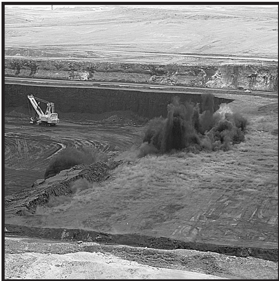
To facilitate mining of a coal seam in Gillette, Wyoming, blasting was used to loosen the coal after the overburden was removed (above). Approximately half a million tons of coal in a seam 80 feet thick was loosened by this single blast.
